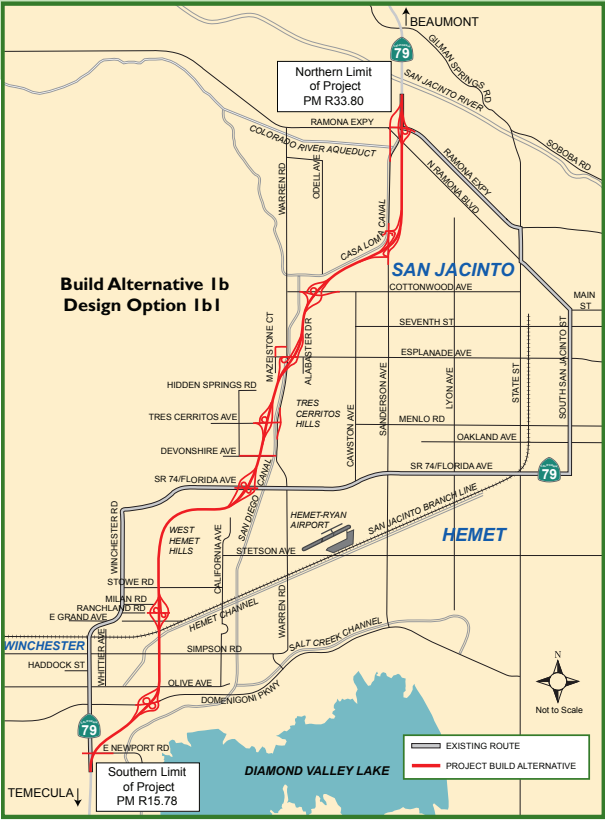
Build Alternative 1b and Design Option 1b1: Starts in the south on Winchester Road and proceeds east to an interchange with Domenigoni, then north on the west side of the West Hemet Hills and then joins the common alignment from Florida to Cottonwood. Design Option 1b1 is on the same alignment but provides a lower roadway profile from Domenigoni to California. In the north, Alternative 1b is closer to Sanderson.
