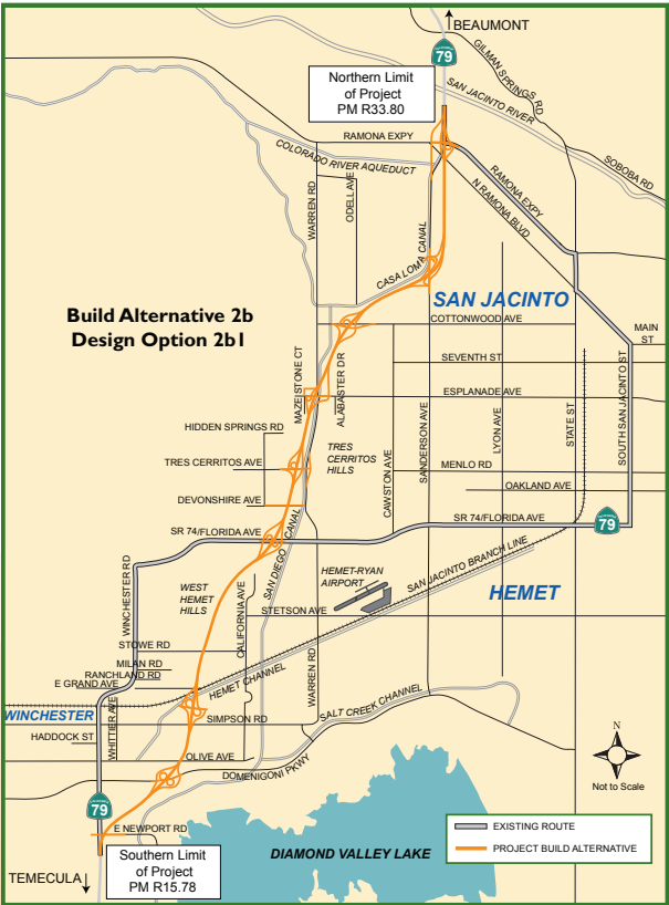
Build Alternative 2b and Design Option 2b1: Starts in the south on Winchester Road and proceeds east to an interchange with Domenigoni, then north through the West Hemet Hills and then joins the alignment from Florida to Cottonwood. Design Option 2b1 is on the same alignment but provides a lower roadway profile from Domenigoni to California. In the north, Alternative 2b is closer to Sanderson.
