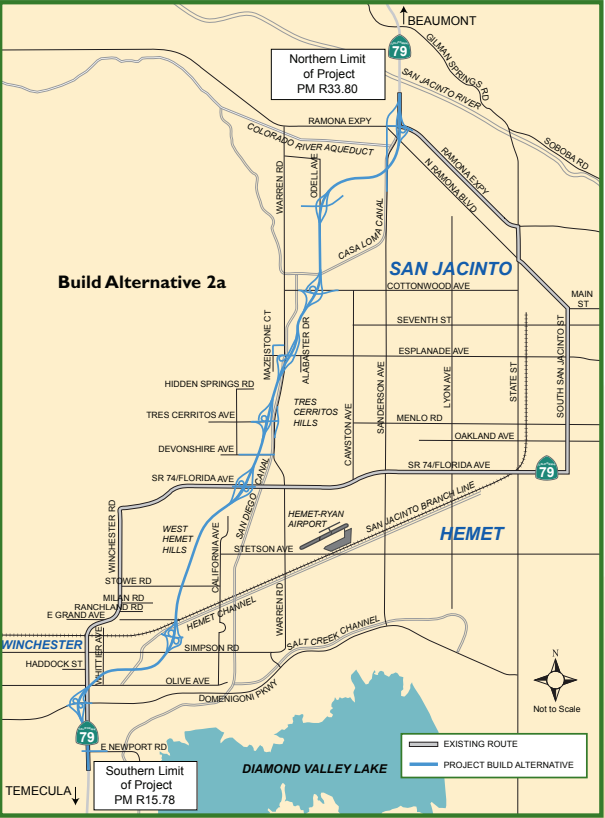
Build Alternative 2a: Starts in the south on Winchester Road, proceeds north through the West Hemet Hills, then joins the alignment from Florida to Cottonwood. In the north, Alternative 2a is closer to Warren.
